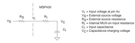
The resistance of the source  $R_S$  and  $R_I$  affect  $t_{sample}$ . The following equation can be used to calculate the minimum sampling time  $t_{sample}$  for a 12-bit conversion:
